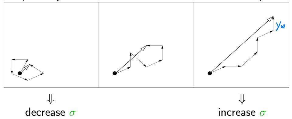
Sampling of solutions, notations as on slide "The  $(\mu/\mu, \lambda)$ -ES - Update of the mean vector" with  ${\bf C}$  equal to the identity.
