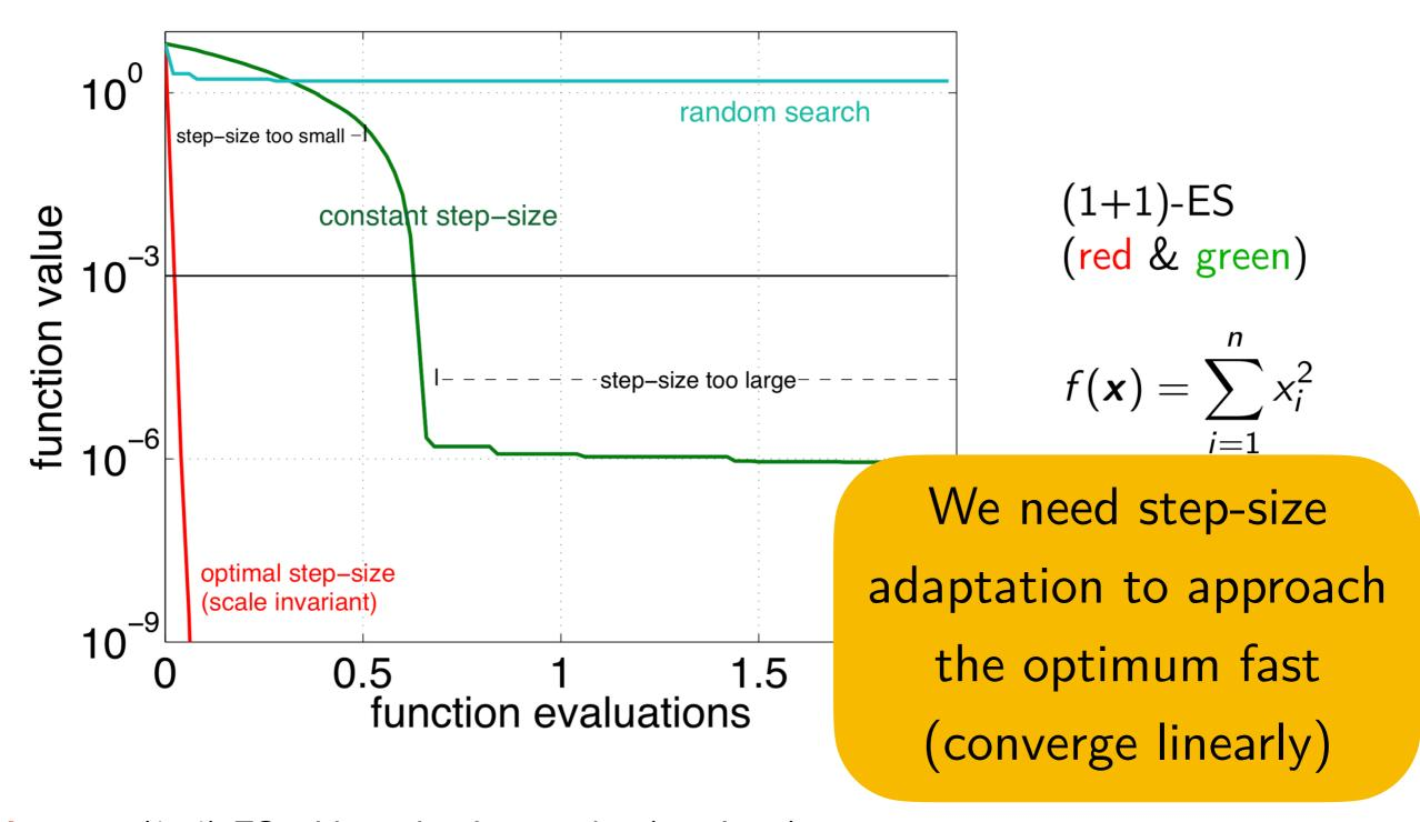
red curve: (1+1)-ES with optimal step-size (see later) green curve: (1+1)-ES with constant step-size ( $\sigma = 10^{-3}$ )
