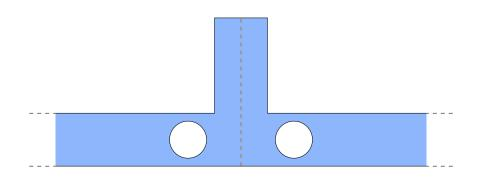
$\blacktriangleright$  We work in waveguides which are symmetric with respect to (Oy) and which contain a branch of finite height.
