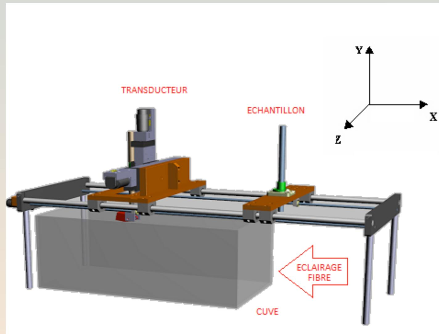
Acoustic detector : transducer (focused at 2cm and 3.5 MHz)
